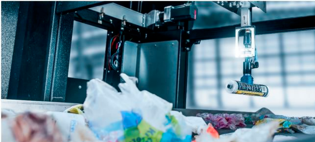
Figure 16. Picker robot in action (Photo: FastPicker, ZenRobotics)
